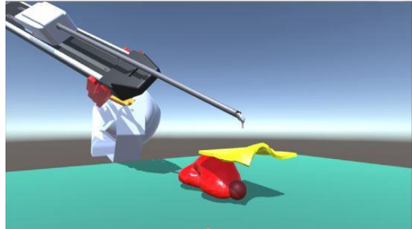
Figure 1. Environment scene developed in Unity3D for robot-assisted nephrectomy procedure. The scene consists of a single PSM arm, kidney, tumour and renal fascia (fat tissue). For visual simplicity, high contrast colours are used to depict various objects
