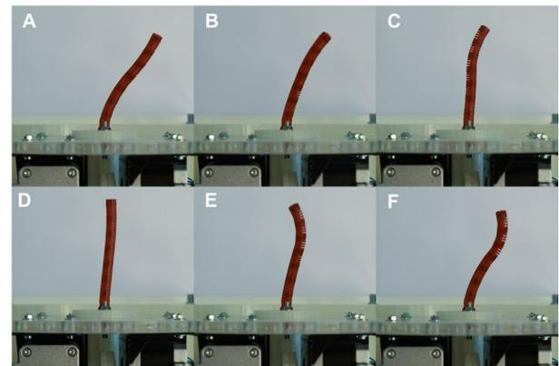
**Figure 4.** Top view of follow-the-leader motions in different steps. From (A) to (C), the leading segment was steered to the right, and followed by the second segment. From (D) to (F), the leading segment was steered to the origin and followed by the second segment.
