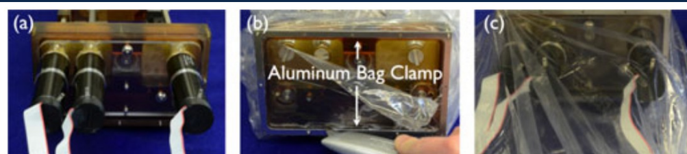
Fig. 3. Sterile barrier concept. (a) Motor plate is removed from the robot before sterilization. (b) Sterile bag is attached to the sterile robot using an aluminum clamp, enabling the motor plate to be subsequently attached and the motors to engage with the Oldham couplings (see Fig. 4). (c) Motor plate is reattached and the bag pulled over it. The robot is now sterile.
